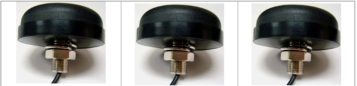
Model#GSM-04A 5-Bands 824-960/1710-1990/2170MHz Gain: 0-1dBi Size: 54.7 x 23.3 (mm) Cable: RG174/U or RG178 *Meets to IP67
