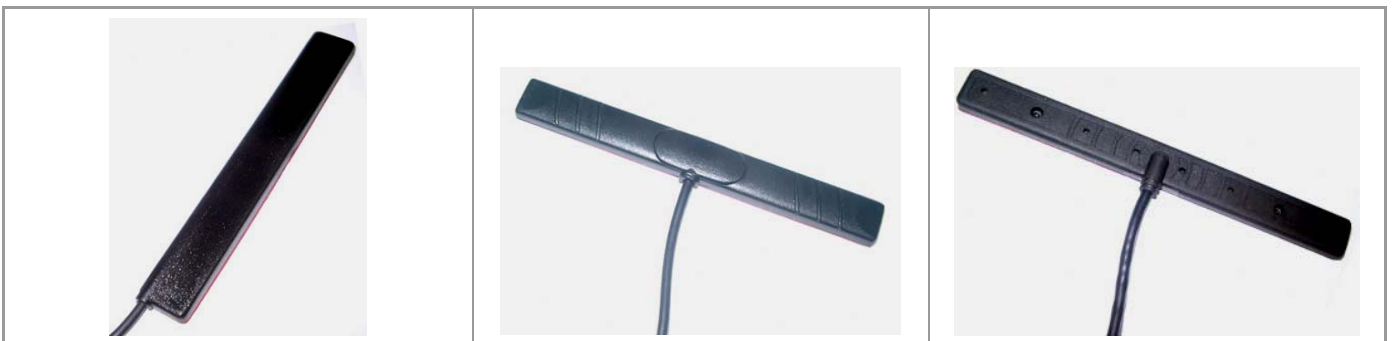
Model#PH-19F (adhesive tape) 5-Bands 824-960/1710-1990/2170MHz Gain: 3dBi Size: 106 x 14.8 (mm) Cable: RG174 A/U
