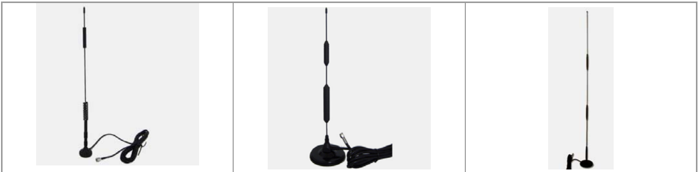
Model#MB-08F 5-Bands+LTE700+LTE2600 700-790/850-960/1710-2170/2690MHz Gain: 5dBi Size: 311.5 x OD29 (mm) Cable: RG174A/U
