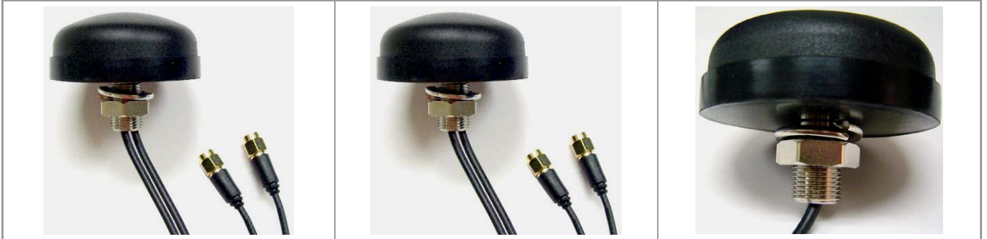
Model#GPS-G04A (Roof) Combo GPS Active + GSM 5 Bands Size: 54.7 x 23.3 (mm) Cable: RG174/U x 2 cables *Meets to IP67
