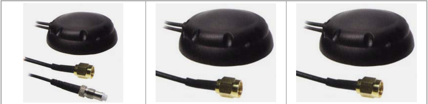
Model#GPS-G01A (Patch Sticker) Combo GPS Active + GSM 5 Bands LNA Gain: 28dB Size: OD50.4 x H17 (mm) Cable: RG174/U x 2 cables
