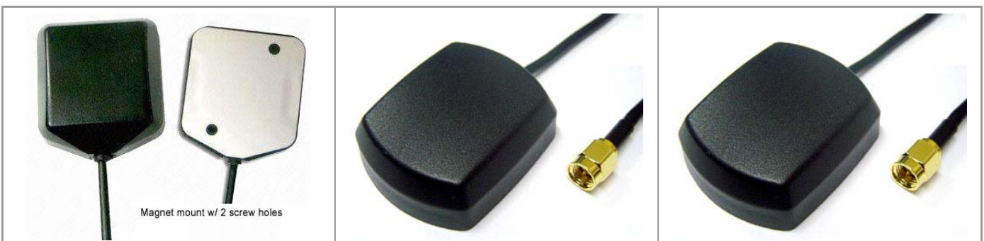
Model#GPS-03A (Magnet w/ 2 screw holes) GPS Active ONLY LNA Gain: 28dB Size: 38.2 x 34.2 x 12.6(mm) Cable: RG174/U
