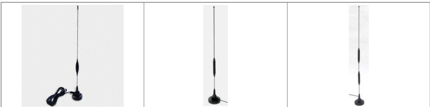
Model#MB-34F 5-Bands 824-960/1710-1990/2170MHz Gain: 5dBi Size: 340.5 x OD40 (mm) Cable: RG174A/U
